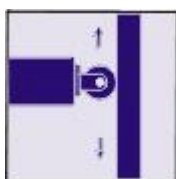
guide pulley and sideway which make lift table's operation more stable
